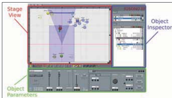
Figure 3. Screenshot of the spatial audio workstation. The three main areas of the user interfaces are shown.
